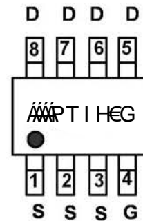
Marking and pin Assignment
